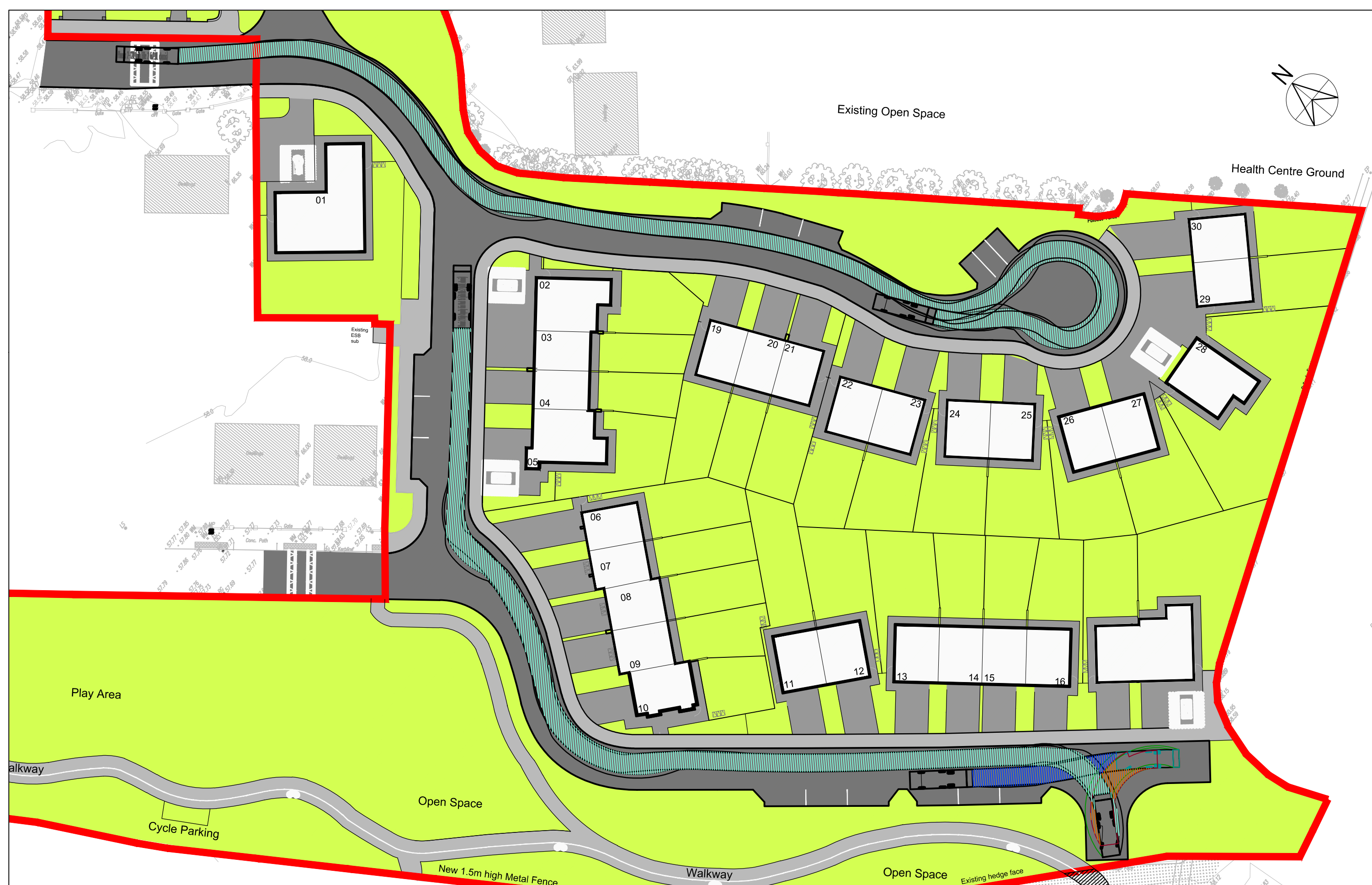
SWEPT PATH ANALYSIS – REFUSE TRUCK SCALE 1:250
